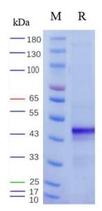
On SDS-PAGE under reducing (R) condition. The gel was stained overnight with Coomassie Blue. The purity of the protein is greater than 90%.
